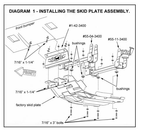
Reinstall the skid plate and tighten all 7/16" hardware (37).
