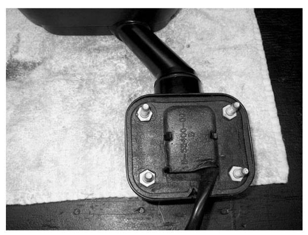
002 Removing motor housing and other parts that fold the mirror.
