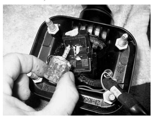
006 Those are magnets on either side, they are for the circuit board sensor to "count" revs, I guess.
