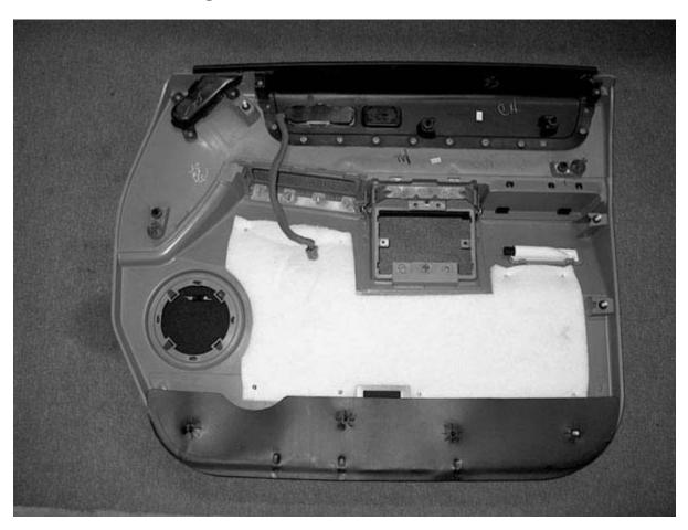
006a What it looks like with panel off. You will want to start pulling the upper right side insulation loose to get to the mirror bolts, I left the window up.
