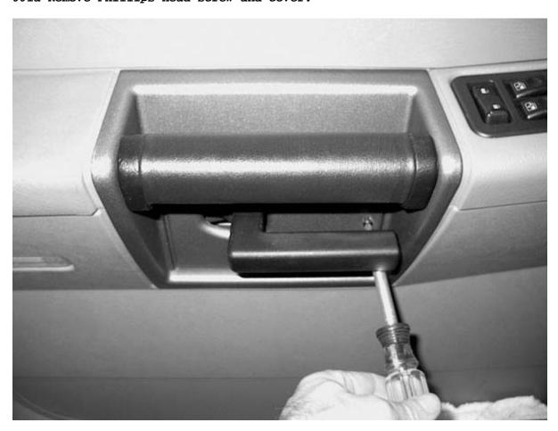
002a Remove two bolts behind cover that was just removed.
