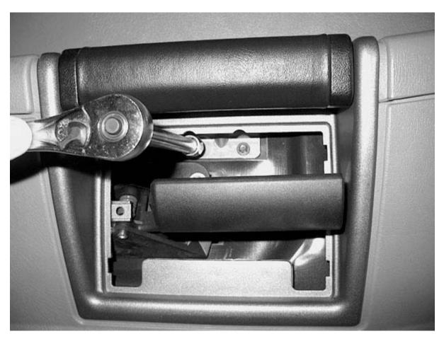
003a Remove button panel. There are four "hooked shaped" areas on the panel, two on each side that need to be "unhooked" from the door panel. I used a putty knife and a rag to protect door panel. The other panel above this one stays in place.
