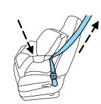
7. Allow the safety belt to retract and remove any slack in the belt to securely tighten the child safety seat in the vehicle.
