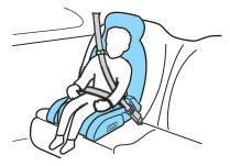
Either type can be used at any seating position equipped with lap/shoulder belts if your child is over 40 lb. (18 kg).
