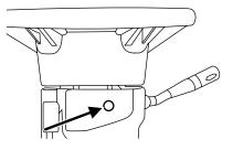
3. Remove the access plug using a flat head screwdriver, then push the override button using a flat head screwdriver, apply the brake pedal and shift the transmission into N (Neutral).
