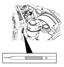
5. Locate and carefully remove the engine oil level indicator (dipstick).6. Wipe the indicator clean. Insert the indicator fully, then remove it again.
