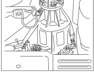
3. Add only enough fluid through the filler opening so that the fluid level is at the bottom of the opening.
