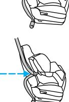
4. Insert the belt tongue into the proper buckle (the buckle closest to the direction the tongue is coming from) for that seating position until you hear a snap and feel the latch engage. Make sure the tongue is latched securely by pulling on it.
