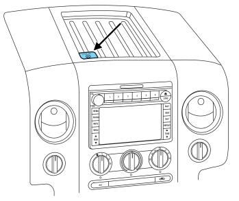
Your vehicle may be equipped with an Auxiliary Input Jack (AIJ), located in the instrument panel tray. The Auxiliary Input Jack provides a way to connect your portable music player to the in-vehicle audio system. This allows the audio from a portable music player to be played through the vehicle speakers with high fidelity. To achieve optimal performance, please observe the following instructions when attaching your portable music device to the audio system.
