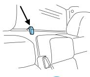
If the tether strap is clipped incorrectly, the child safety seat may not be retained properly in the event of a collision.
