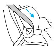
8. Allow the safety belt to retract to remove any slack in the belt.
