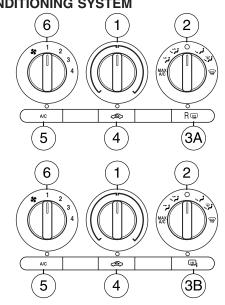
3. A. **R** Rear defroster (if equipped): Press to defrost the rear window. Refer to *Rear window defroster (if equipped)* later in this chapter for more information.
