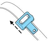
4. While holding both shoulder and lap portions next to the tongue, route the tongue and webbing through the child seat according to the child seat manufacturer's instructions. Be sure that the belt webbing is not twisted.
