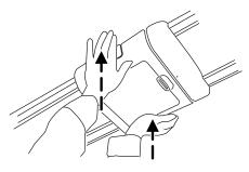
While pushing upwards with palms, grip the side latches with fingers and squeeze.
