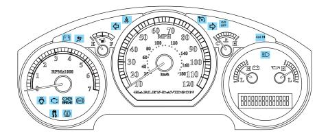
Warning lights and gauges can alert you to a vehicle condition that may become serious enough to cause expensive repairs. A warning light may illuminate when a problem exists with one of your vehicle's functions. Many lights will illuminate when you start your vehicle to make sure the bulb works. If any light remains on after starting the vehicle, refer to the respective system warning light for additional information.
