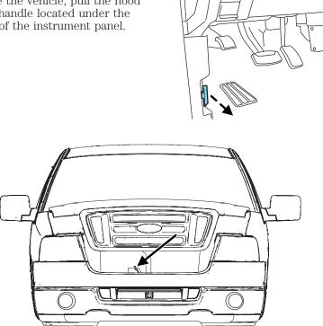
2. Go to the front of the vehicle and release the auxiliary latch that is located on the front bumper under the grill.
