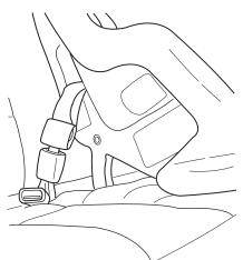
• LATCH lower anchors are recommended for use by children up to 22 kg (48 pounds) in a child restraint. Top tether anchors can be used for children up to 27 kg (60 pounds) in a child restraint, and to provide upper torso restraint for children up to 36 kg (80 pounds) using an upper torso harness and a belt-positioning booster.
