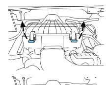
2. Pull air filter tray assembly out toward front of vehicle and lift air filter element up and out of housing.
