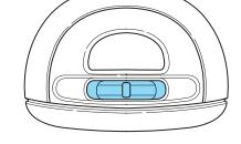
With the ignition key in the ACC or ON position, the rear dome lamp can be turned ON or OFF by sliding the control.
