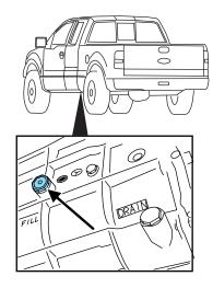
2. Remove the filler plug and inspect the fluid level.
