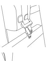
shortened, but pinches the webbing to keep the lap portion from getting longer. The cinch tongue is designed to slip during a crash, so always wear the shoulder belt properly and don't allow any slack in either the lap or shoulder portions.
