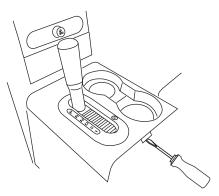
4. Press and hold the white button located along side the shifter housing assembly (as shown in the illustration). Press the gearshift lever release on the shifter knob and move the gearshift lever back to N (Neutral) (two places rearward from P [Park]).
