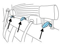
and as an anchoring loop for child seats installed in the outboard rear seats.
