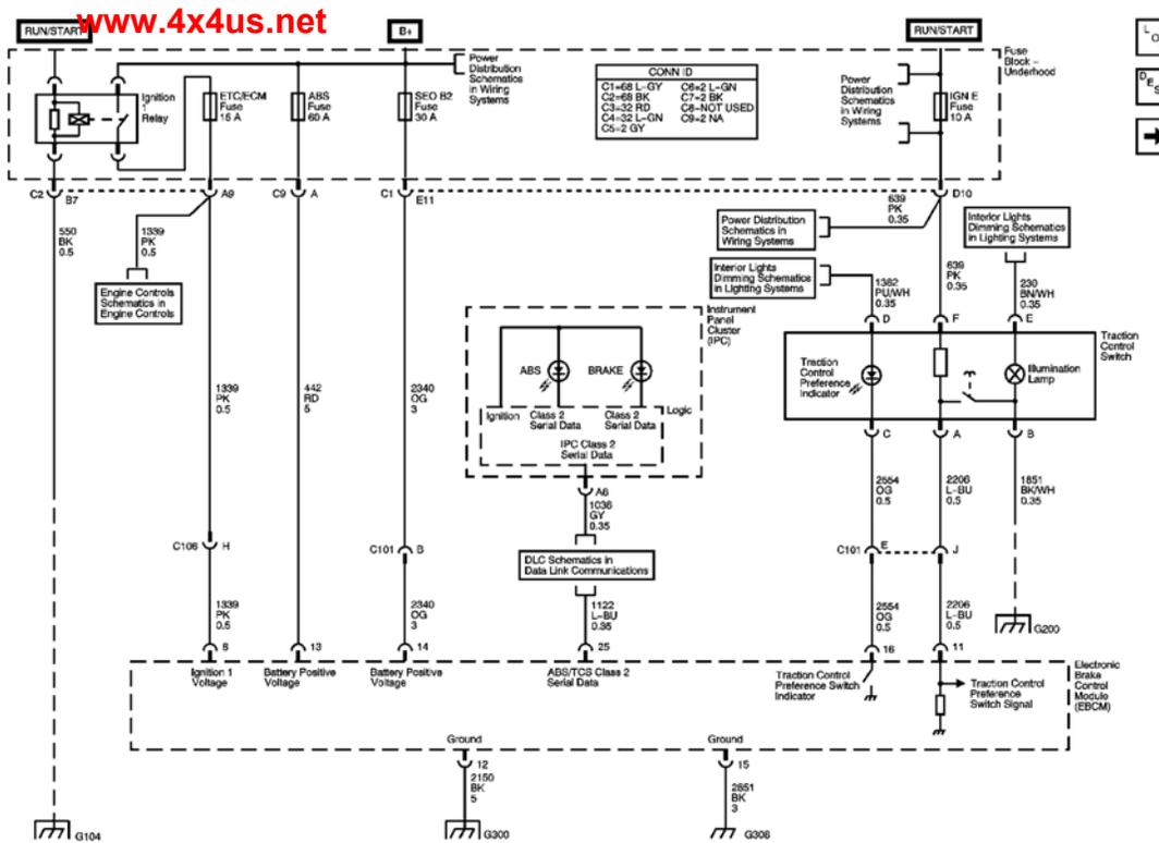
**Fig. 1: EBCM Power, Ground, DLC, Indicator Lamps, and Traction Control Switch**
