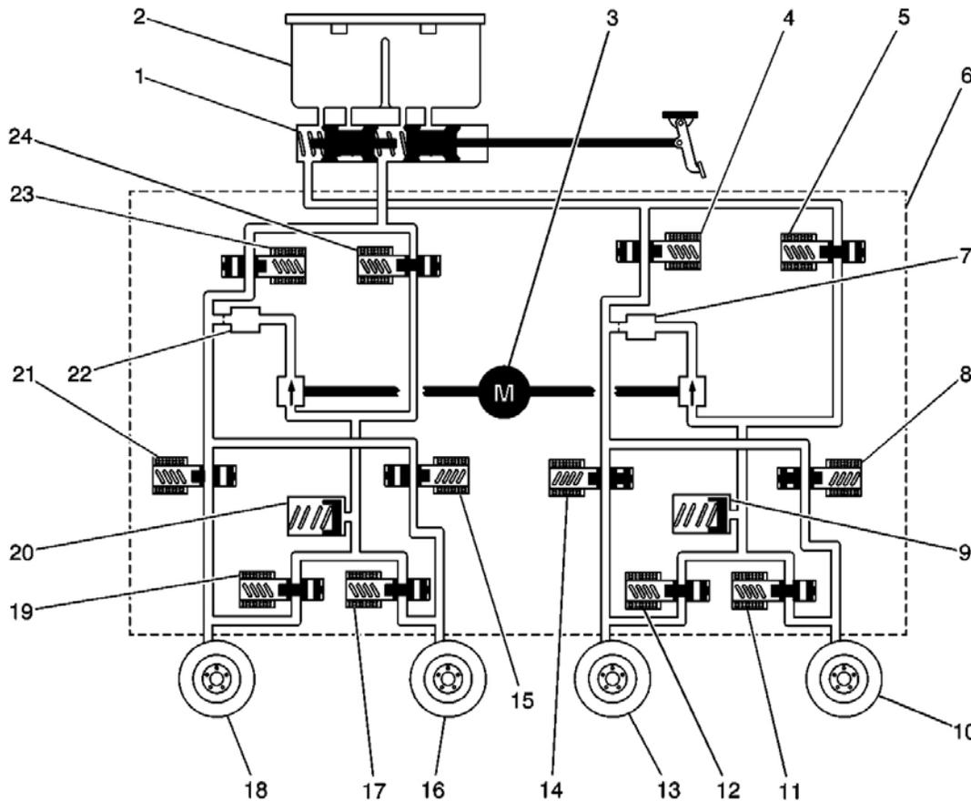
**Fig. 24: BPMV Hydraulic Flow**
