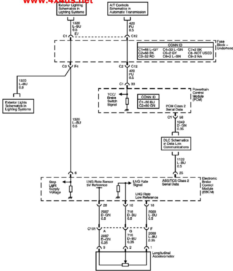
**Fig. 2: Stoplamp Switch and Longitudinal Accelerometer Inputs**
