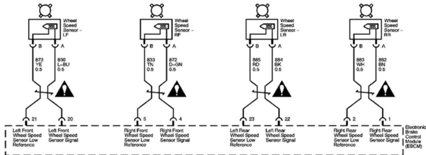
**Fig. 3: Wheel Speed Sensor Inputs**
