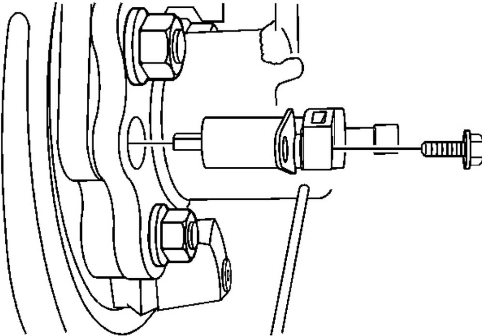
**Fig. 18: Rear Wheel Speed Sensor & Shim**
