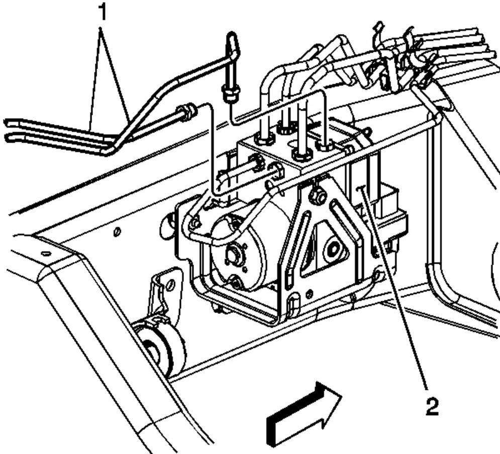
**Fig. 8: Rear Brake Pipes & BPMV**
