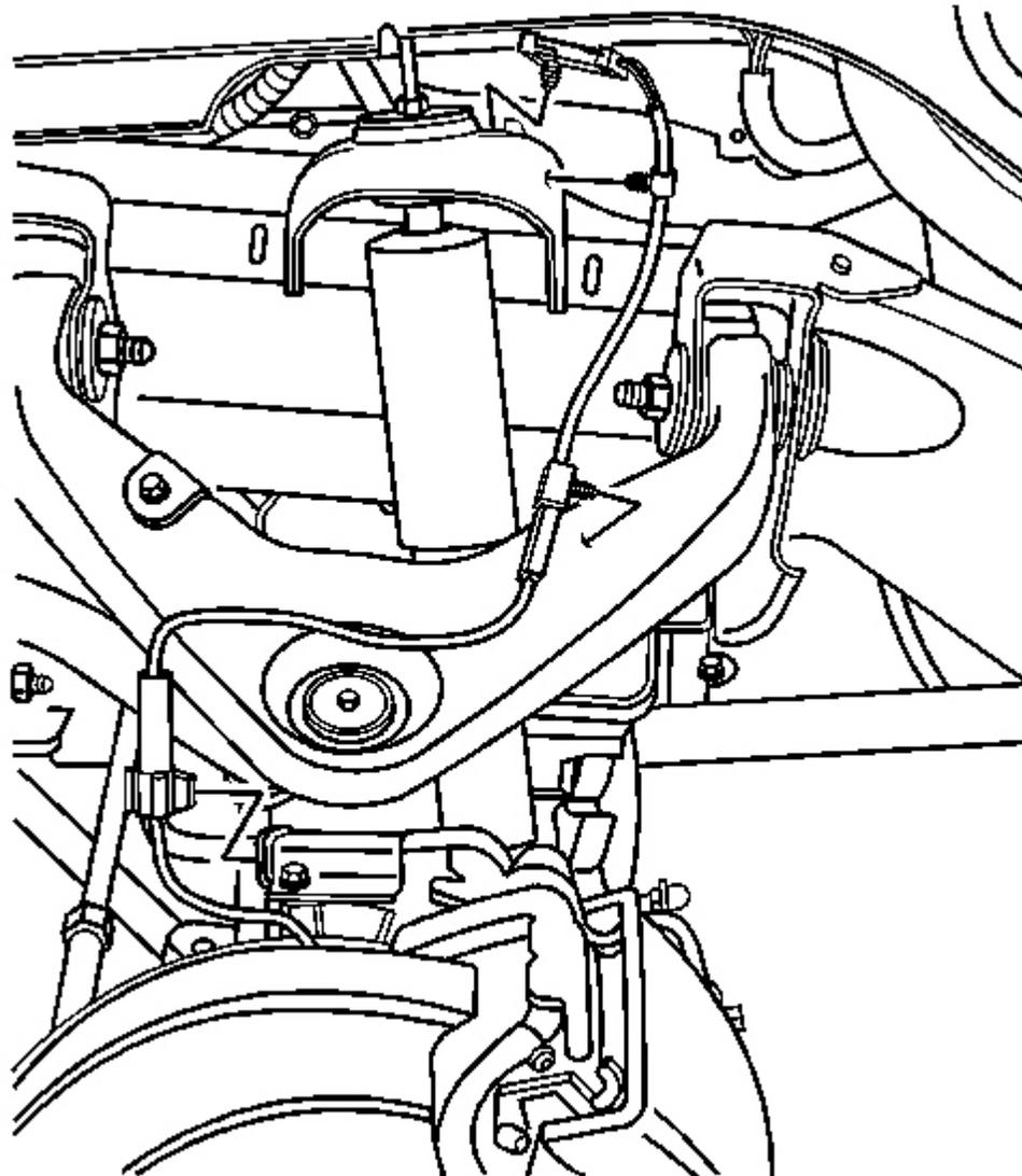
**Fig. 16: Front Wheel Speed Sensor Cable**
