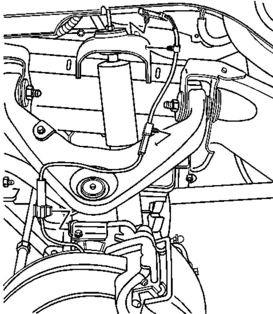
**Fig. 13: Front Wheel Speed Sensor Cable**
