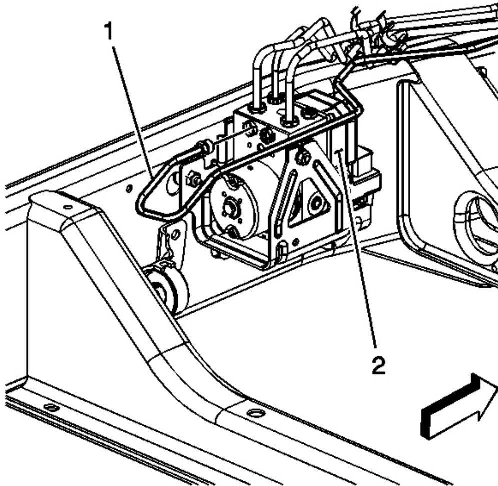
**Fig. 7: Right Front Brake Pipe & BPMV**
