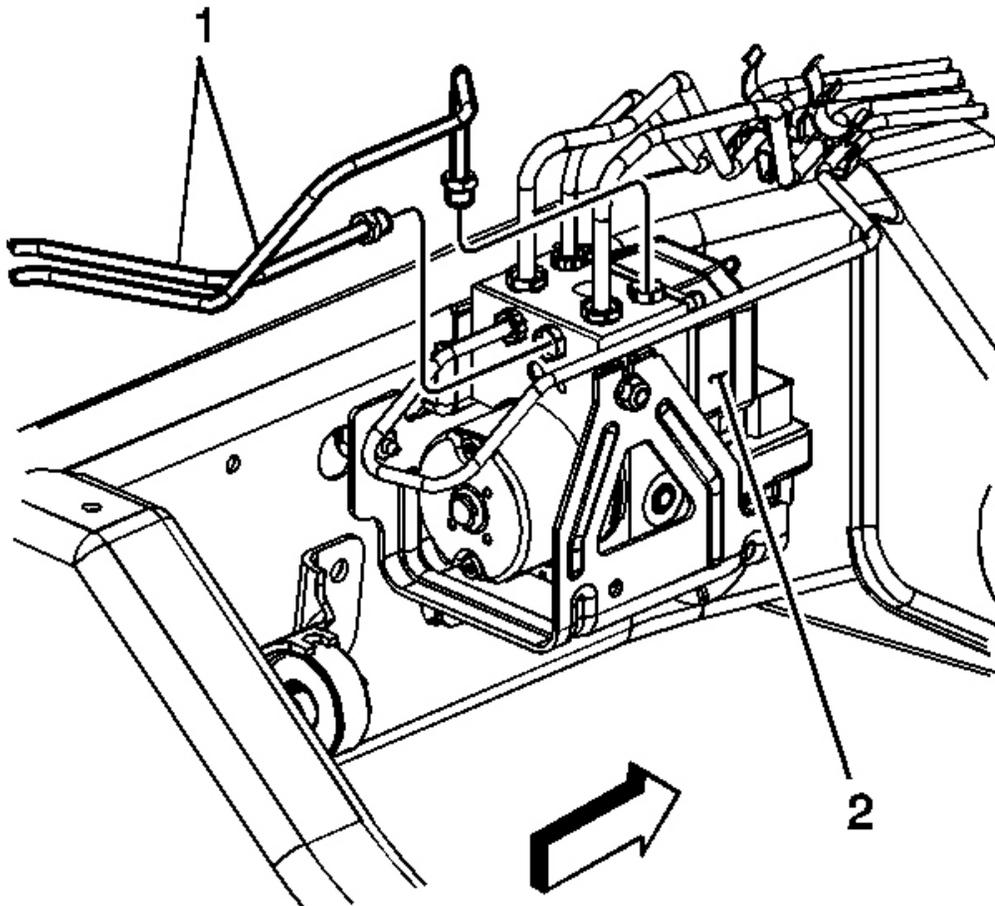
5. Connect the rear brake pipes (1) to the BPMV (2).
