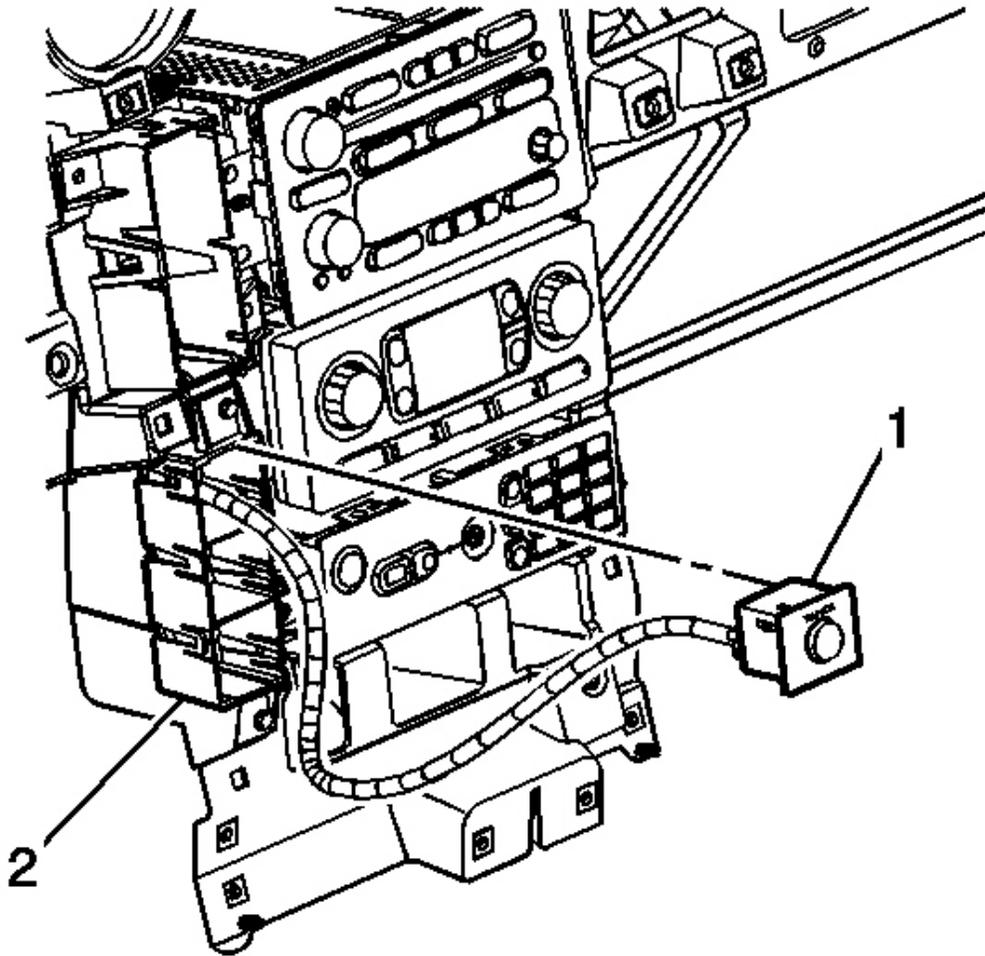
**Fig. 19: Traction Control Switch & I/P Assembly**
